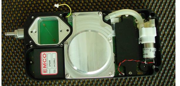
A photograph of the miniDiSC instrument with the wire-mesh screen removed. The wire-mesh screen is a green mesh component that has been lifted off and is placed to the left of the main instrument. The instrument's internal components are visible, and the yellow cable is now disconnected from the top of the instrument.                                           |
