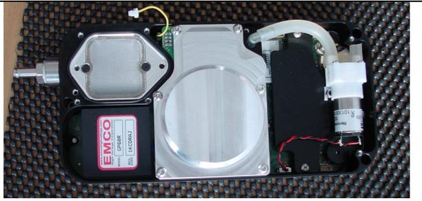
A photograph of the miniDiSC instrument with the counterelectrode removed. The counterelectrode is a white plastic component that has been lifted off and is placed to the left of the main instrument. The instrument's internal components are visible, and the yellow cable is now disconnected from the top of the instrument.                                         |
